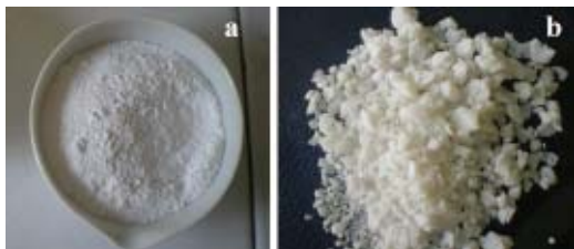
Fig. 3. Optical images of the hydroxyapatite (a) and nanohydroxyapatite - calcium fructoborate biocomposite (b)
